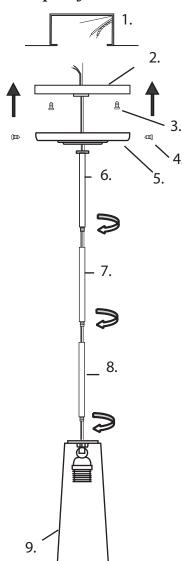
\*\*\*DETERMINE REQUIRED MEASUREMENT BEFORE MAKING CONNECTION-IT MAYBE NECESSARY TO REMOVE SOME OF THE RODS TO OBTAIN THE DESIRED LENGTH\*\*\*
